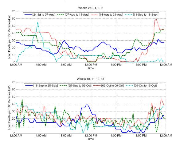
Figure 9: Aggregate Load Profile Based on Real-World Field Test Charge Scenario Data
