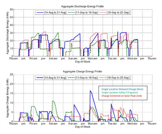
Figure 8: Charge and Discharge Aggregate Capacities of the Test Fleet during Weeks 5, 9, and 10
