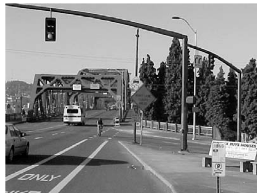
Bicycle lanes alert merging drivers on the approach to the Broadway Bridge to where bicyclists will be
