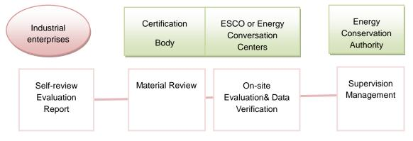
Figure 13: The General Evaluation Procedures for Energy Performance Evaluation
