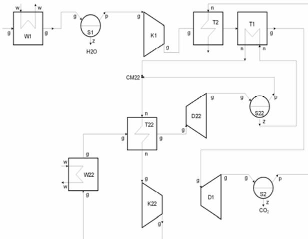
Figure 4. System for CO<sub>2</sub> removal: W1, W22 – gas-water heat exchanger, K1 – compressor of combustion products, K22 – compressor of nitrogen refrigerating cycle, S1, S2, S22 – liquid phase separators, T1 – a group of regenerative coolers, T2 – a group of coolers using external cooling agent, T22 – a group of coolers in the nitrogen cooling cycle, D1, D22 – turbine expanders.
