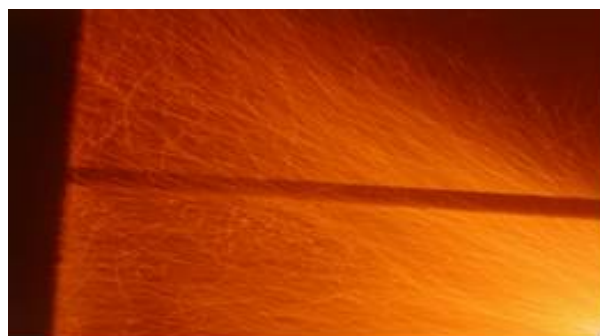
Fig.2. The torch in the furnace volume of the heat-and-power test-bench at brown coal combustion in the vibrocentrifugal mill.
