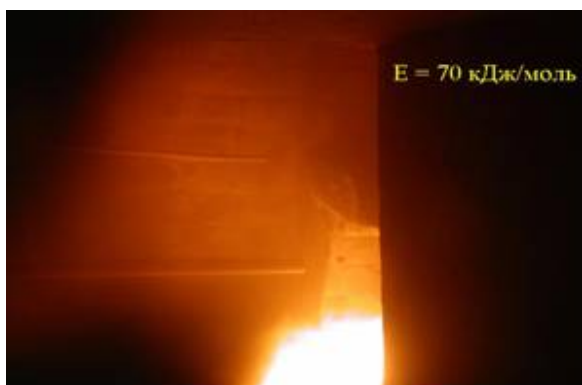
Fig.3. Coal and dust torch burning at mechanically activated microgrinded coal in the disintegrating mill.
