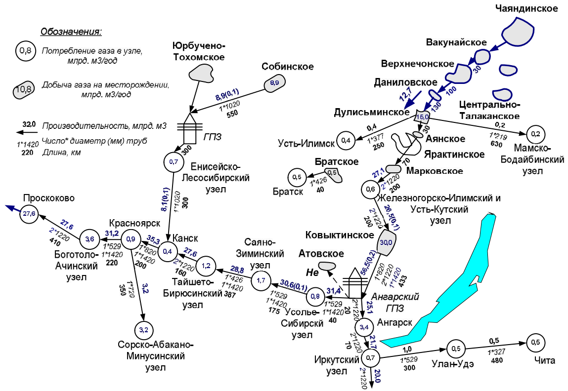
Figure. Calculated scheme of gas supply of the Siberian Federal District for 2030
