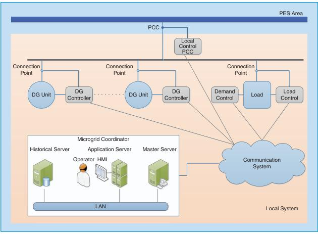
figure 7. Communications architecture of a microgrid.
