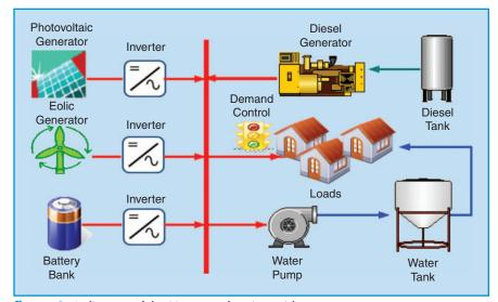
figure 8. A diagram of the Huatacondo microgrid.
