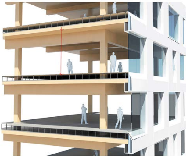
East-West Section showing engineered plenum
