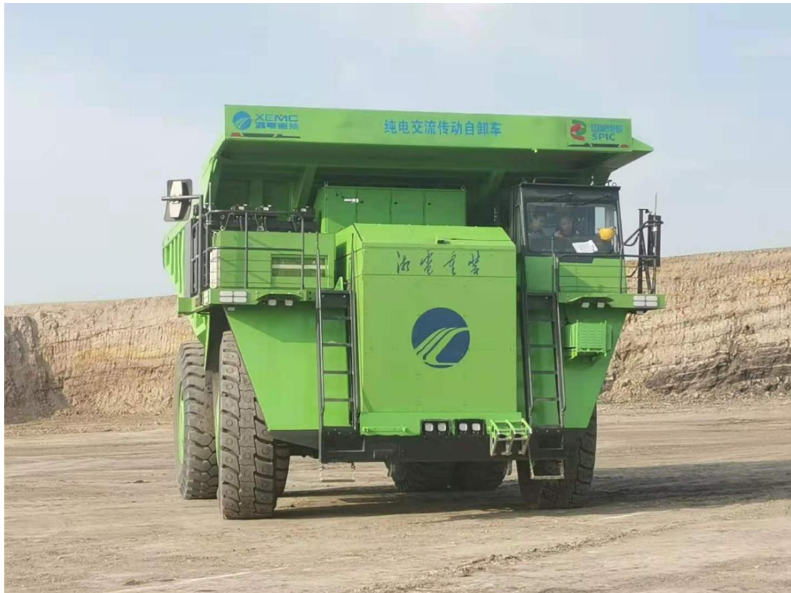
Figure 13. Pure Electric Power Self-unloading Mining Truck of 120 Tone Load on the Scene
