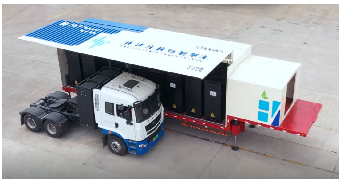
Figure 5. SPIC Mobile Battery-Swap Vehicle (Trailer)
